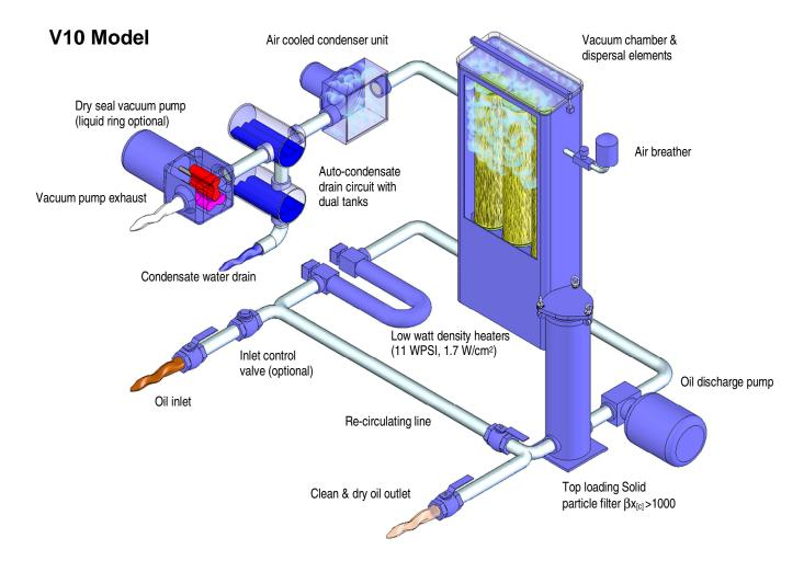
The dehydrated oil flows to the bottom of the vacuum chamber and is removed by the discharge pump. The oil is pumped through the high efficiency particulate filter assembly ( $\beta x_{[c]} > 1000$ ) and returned to the system. The re-circulating line helps the VAC-U-DRY reach optimum temperature in cold start situations and can be used to throttle machine inlet and outlet flow.
